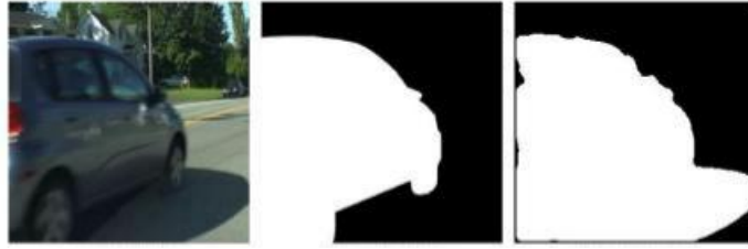
Figure 1. From left to right: input video sequence frame, ground-truth segmentation, and segmentation result from an existing method. The shadow is erroneously segmented along with the vehicle.
